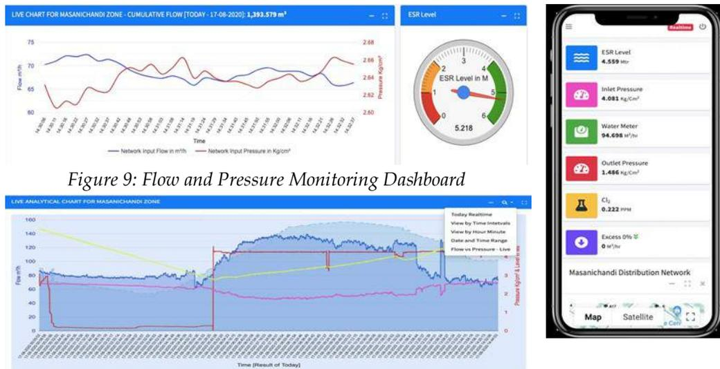
Figure 9: Flow and Pressure Monitoring Dashboard
